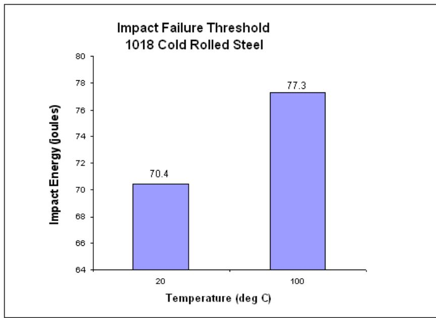
Table 2. Impact failure threshold of 1018 cold rolled steel
